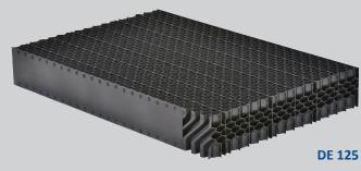
Small and medium size cooling towers demand efficient drift eliminator systems to significantly reduce water losses caused by upstreaming air above the cooling fill. These film drift eliminator elements are easy to install and can be dismantled and cleaned for further use in the cooling tower.
