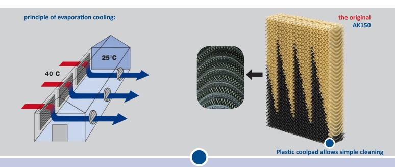
The original **HEWiCOOL PAD** supports a continuous controlled climate cased by a cool stable air temperature and optimal humidity at higher outdoor temperatures.
